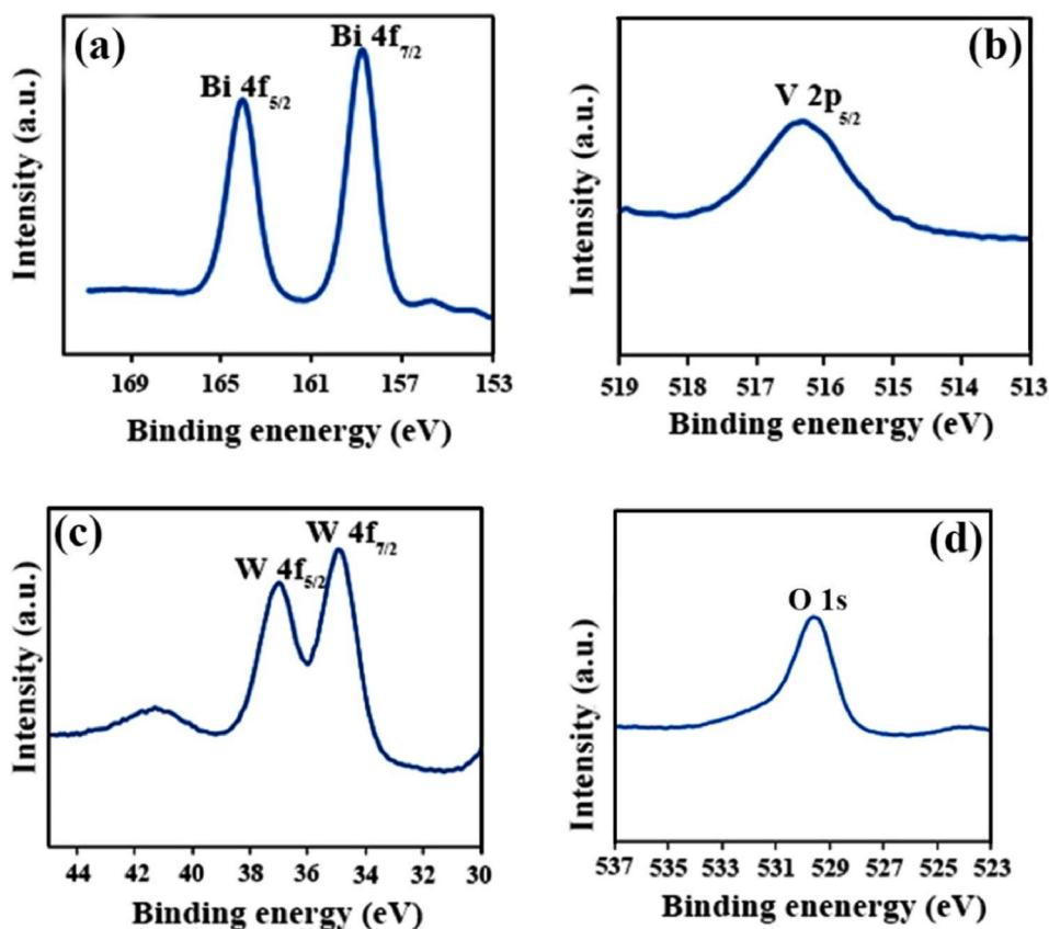
**Fig. 4.** XPS spectra of (a) Bi 4f, (b) V 2p, (c) W 4f, and (d) O 1s on FTO/ $\text{WO}_3/\text{BiVO}_4$  electrode fabricated by dip coating technique.
