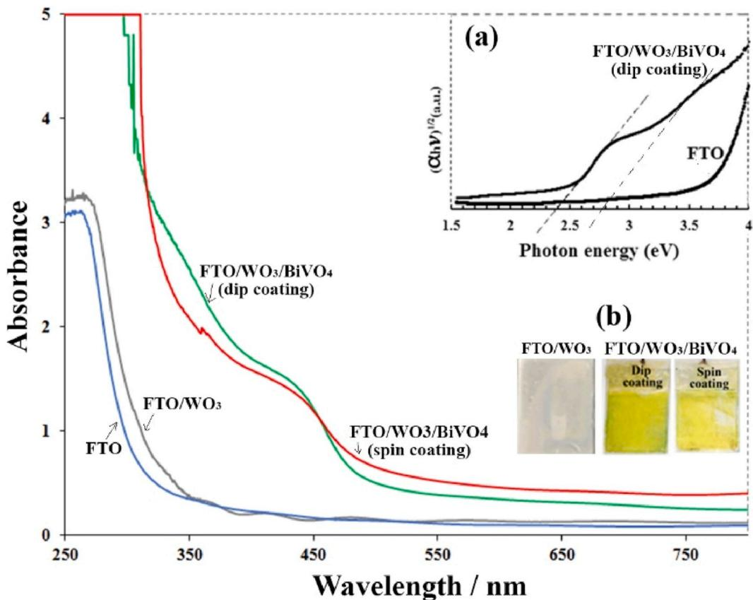
**Fig. 2.** UV/Vis absorption spectra of FTO substrate, FTO/WO<sub>3</sub>, and FTO/WO<sub>3</sub>/BiVO<sub>4</sub> prepared by dip coating and spin coating techniques. Inset of (a) shows the correlation between the absorbance coefficient and bandgap energy of FTO and FTO/WO<sub>3</sub>/BiVO<sub>4</sub> prepared by dip coating technique and (b) shows the colour of FTO/WO<sub>3</sub> and FTO/WO<sub>3</sub>/BiVO<sub>4</sub> thin film prepared by spin coating and dip coating techniques.
