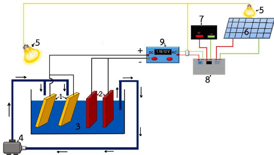
**Fig. 1.** Schematic PEC cell design including solar cell system (1) FTO/WO<sub>3</sub>/BiVO<sub>4</sub> anode electrode, (2) stainless steel cathode electrode, (3) organic dyes solution, (4) pump, (5) light sources, (6) solar cell, (7) battery, (8) circuit board, and (9) voltage control panel.
