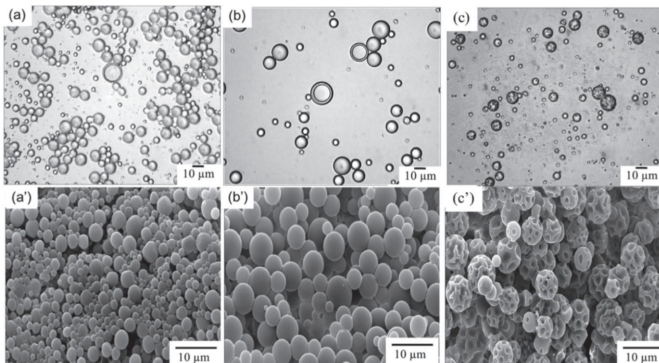
**Figure 5.** Optical (a) – (c) and SEM (a') – (c') micrographs of P(MMA-co-EGDMA)/MA prepared by *ms* ITP with 20 wt% of various kinds of emulsifiers relative to MA: (a), (a') Span 80; (b), (b') oleic acid; (c), (c') DPHS.
