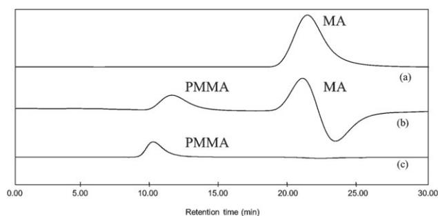
**Figure 2.** GPC chromatograms of MA (curve (a)), PMMA/MA microcapsules (lower layer) (curve (b)) and aqueous dispersion (upper layer) (curve (c)) prepared by *ms* CRP (entry 1).
