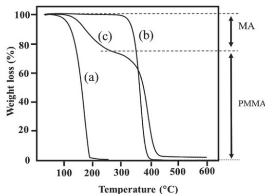
**Figure 4.** TGA thermograms (scanning rate 5 °C min<sup>-1</sup>) of MA (curve (a)), PMMA particles (curve (b), entry 5) and PMMA/MA microcapsules (curve (c), entry 4) prepared by *ms* ITP. The dashed lines are a guide only to estimate the two steps of weight loss of PMMA/MA microcapsules.
