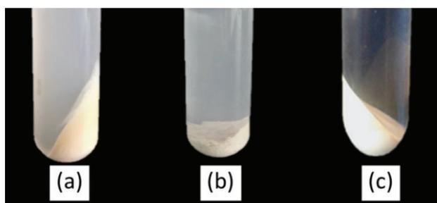
**Figure 3.** Photographs of aqueous dispersions after centrifugation of samples prepared by *ms* ITP at various  $CH_3I$  concentrations (wt% of monomer): (a) 0.2 (entry 2); (b) 0.4 (entry 3); (c) 0.8 (entry 4).
