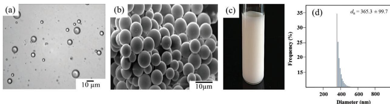
**Figure 1.** (a) Optical and (b) SEM micrographs and (c) suspension photograph of PMMA/MA microcapsules prepared by *ms* CRP (entry 1); (d) dynamic light scattering histogram of the number-average diameter ( $d_n$ ) of polymer particles in aqueous phase after centrifugation at 8000 rpm.
