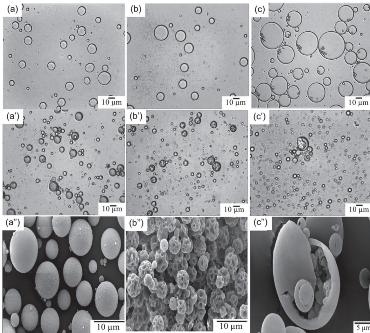
**Figure 6.** Optical micrographs of monomer droplets (a)–(c) and P(MMA-*co*-EGDMA)/MA microcapsules (a')–(c') and SEM micrographs of P(MMA-*co*-EGDMA)/MA microcapsules (a'')–(c'') prepared by *ms* ITP at various concentrations of DPMS (wt% relative to MA): (a), (a'), (a'') 10 (entry 12); (b), (b'), (b'') 20 (entry 13); (c), (c'), (c'') 30 (entry 14).
