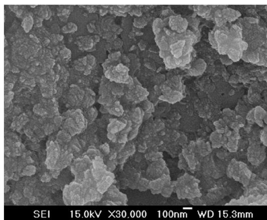
Fig. 2. SEM image of  $\text{CaO}_2$  after drying at  $80^\circ\text{C}$ .
