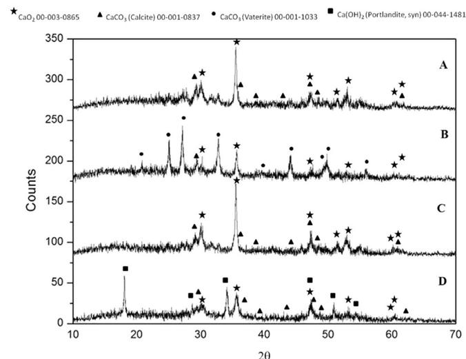
Fig. 1. XRD patterns of the products prepared using Ca(NO<sub>3</sub>)<sub>2</sub> as a precursor under various conditions after drying at 80 °C.
