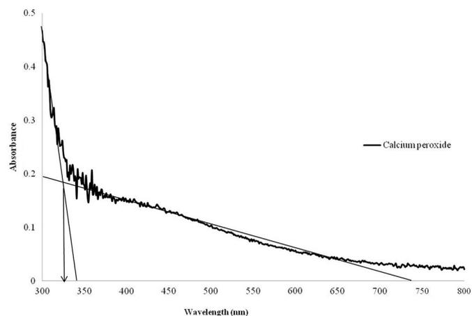
Fig. 5. UV-Vis diffuse reflectance spectrum of  $\text{CaO}_2$ .
