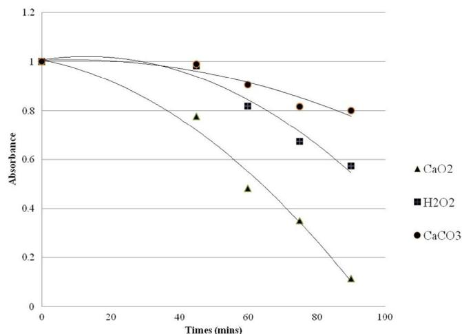
Fig. 4. Photooxidation activity of  $\text{CaO}_2$  under visible light comparison between  $\text{CaO}_2$ ,  $\text{H}_2\text{O}_2$  and  $\text{CaCO}_3$ .
