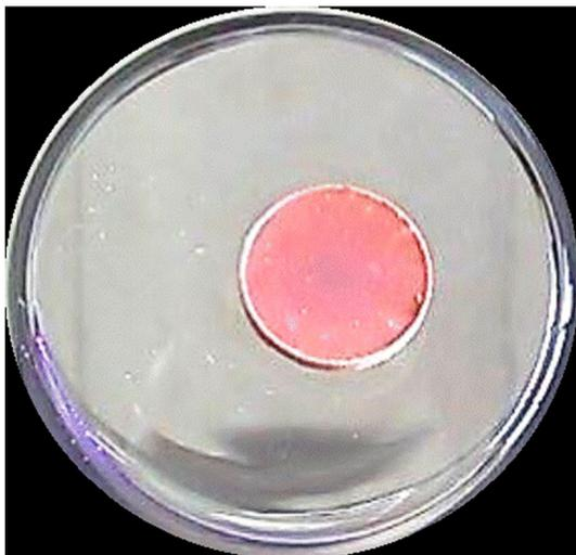
Fig. 6. Photoreduction of resazurin of  $\text{CaO}_2$  under visible illumination.
