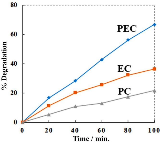
Fig. 10. % Methylene blue dye degradation using photocatalytic (PC), electrocatalytic (EC), and photoelectrocatalytic (PEC) mechanisms.
