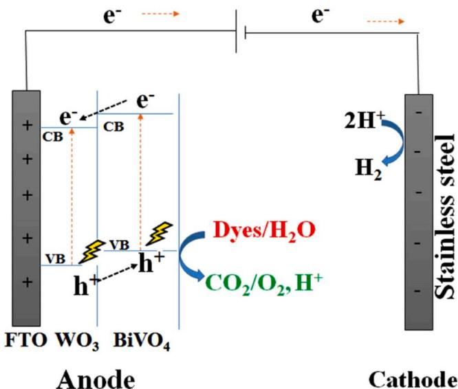
Fig. 11. Schematic diagram of FTO/WO<sub>3</sub>/BiVO<sub>4</sub> photoanode electrode for dyes degradation under the photoelectrocatalytic mechanism.
