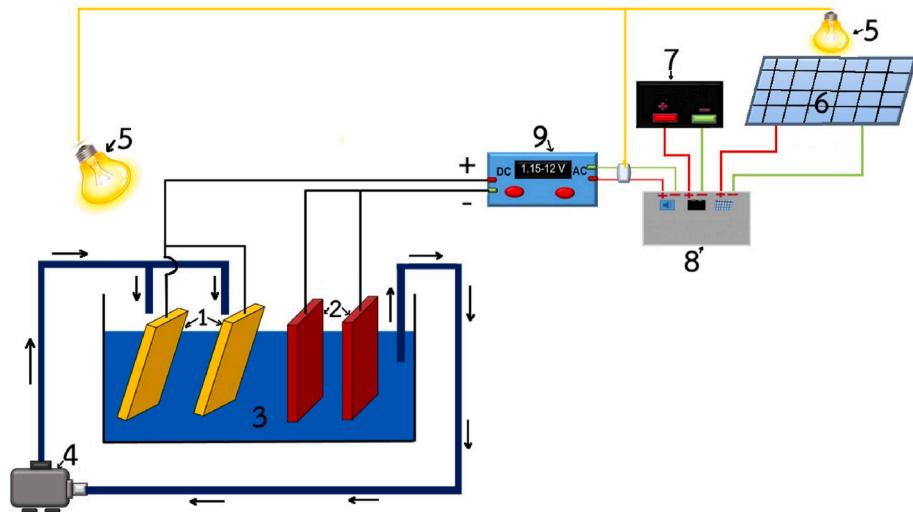
**Fig. 1.** Schematic PEC cell design including solar cell system (1) FTO/WO<sub>3</sub>/BiVO<sub>4</sub> anode electrode, (2) stainless steel cathode electrode, (3) organic dyes solution, (4) pump, (5) light sources, (6) solar cell, (7) battery, (8) circuit board, and (9) voltage control panel.
