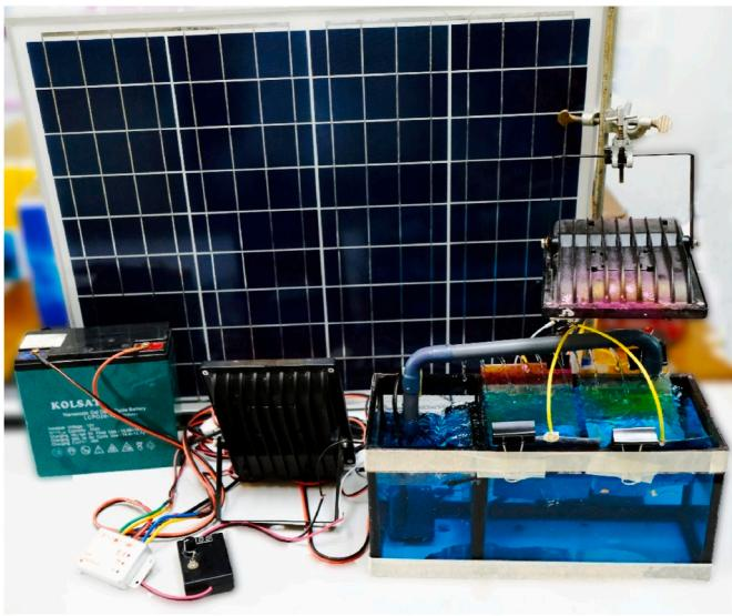
**Fig. 7.** Experimental set up of the designed PEC cell for dye degradation process.
