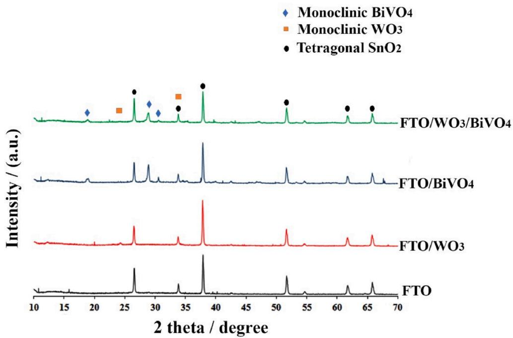
**Fig. 5.** X-ray diffraction patterns of FTO substrate, FTO/WO<sub>3</sub>, FTO/BiVO<sub>4</sub> and FTO/WO<sub>3</sub>/BiVO<sub>4</sub> prepared by dip coating techniques.
