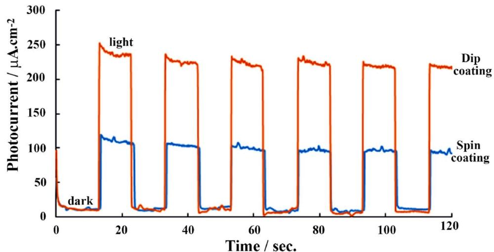
**Fig. 6.** Photocurrent of FTO/WO<sub>3</sub>/BiVO<sub>4</sub> electrode with different fabrication of dip coating and spin coating techniques at 1.0 V vs. Ag/AgCl in 0.1 M Na<sub>2</sub>SO<sub>4</sub> aqueous solution under periodical visible light irradiation.
