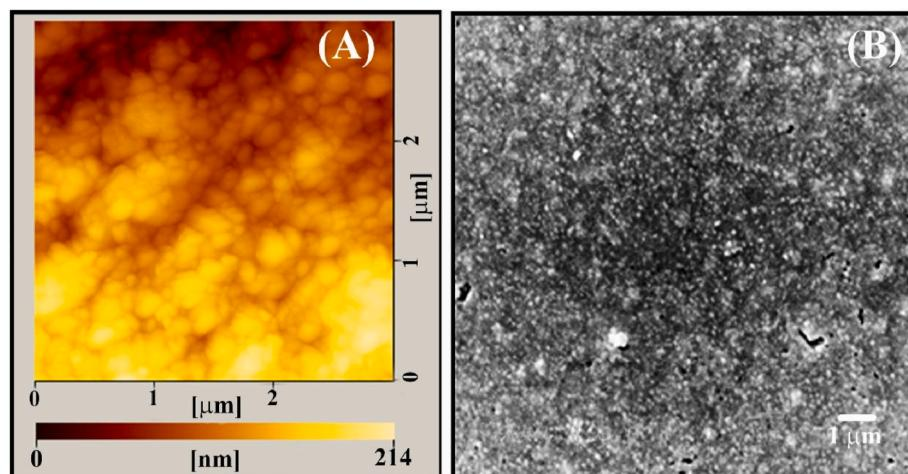
**Fig. 3.** (A) AFM images and (B) SEM image on the top sectional view images of the fabricated  $\text{WO}_3/\text{BiVO}_4$  thin film on FTO substrate using dip coating technique.
