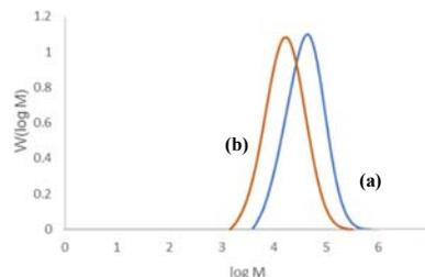
Fig. 2 Molecular weight distribution of PLLA (Mw 145,000) after glycolysis at various times (min): (a) 30 and (b) 60
